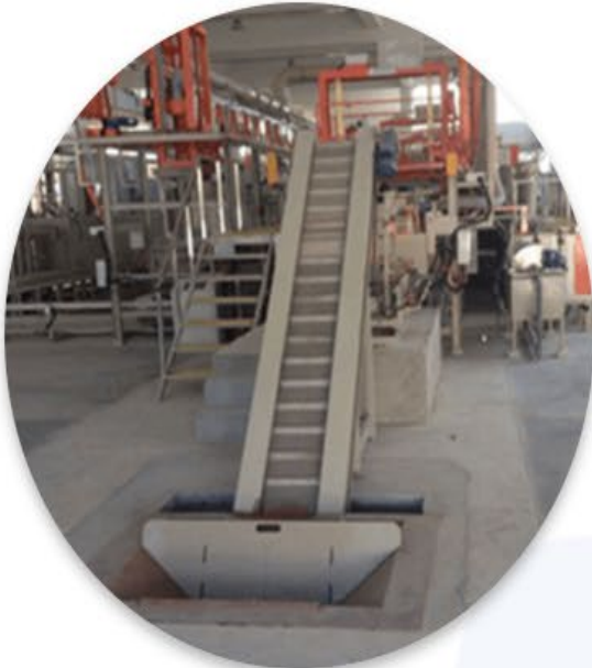
Alkaline Based Zinc Plating Line with on line Hydrogen De-embrittlement
